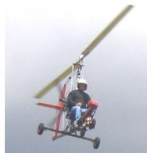
Gyroplane is a rotorcraft that uses rotorblades as a spinning wing to provide lift. Unlike a helicopter the rotorblades are not powered directly by the engine.
